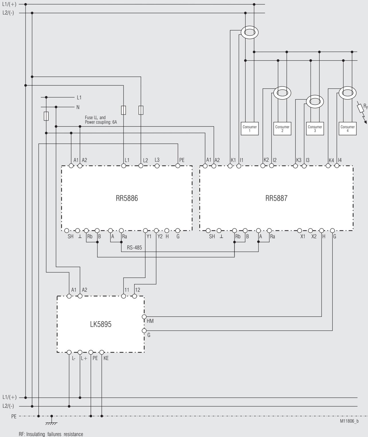
Insulation monitoring and insulation fault detection with 4 connected current transformers in a AC (DC) - network with subdistribution - insulation fault detection can be controlled by the insulation monitor /LK 5895); bus termination of the first and last device on the RS-485 bus.
