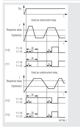
On model MK 9053N/6\_ \_ with manual reset the contacts remain in the fault state after detecting a fault or after to has elapsed. The contacts are reset by disconnecting the supply voltage.
