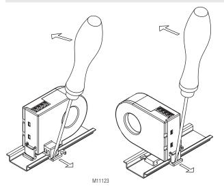
Disassembling Residual Current Monitor ND 5015/070
