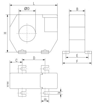
For DIN rail mounting or screw mounting
