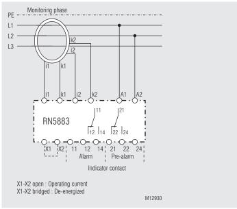
Monitoring of a three-phase network without neutral conductor
