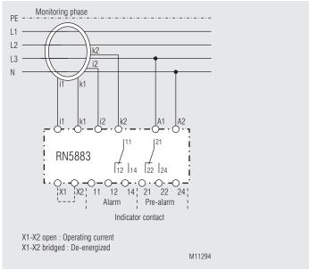
Monitoring of a three-phase network with neutral conductor
