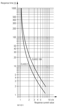
Trigger characteristics Motor overload protection
