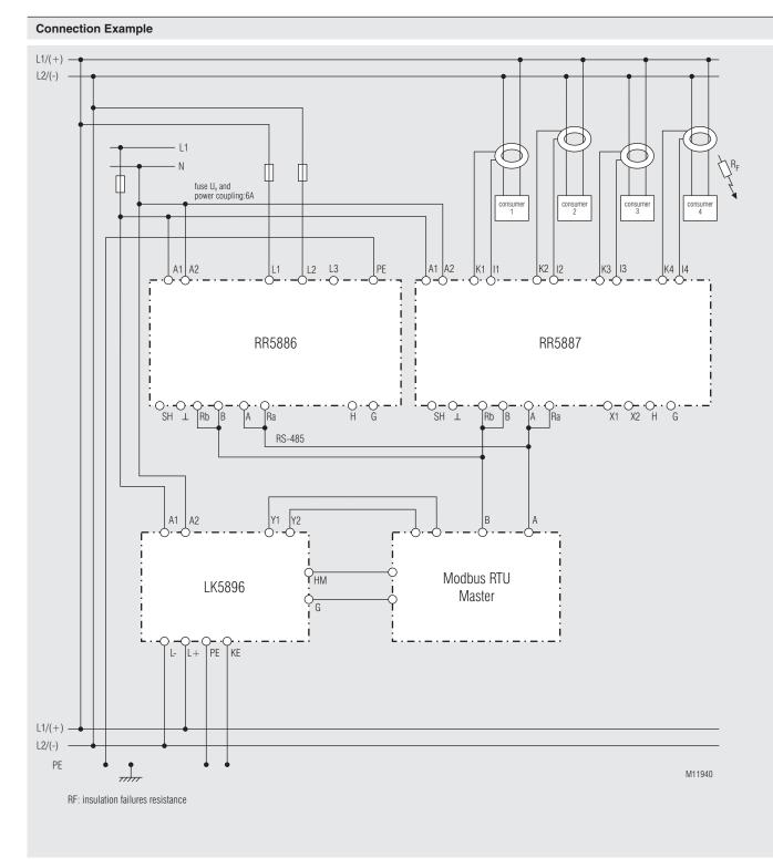
Insulation fault location via Modbus control with external master.
