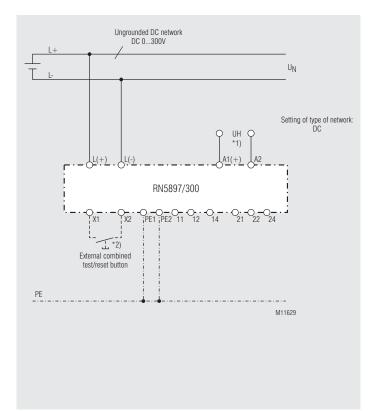
\*1) Auxiliary voltage U<sub>H</sub> (A1(+)/A2) ) can also be sourced from the monitored voltage system. The voltage range of the auxiliary supply has to be taken into account.
