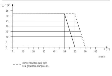
device mounted without distance heated by devices with same load.
