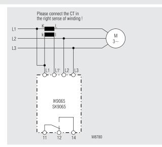
IK/SK 9065.11 with 3-phase load and external current transformer
