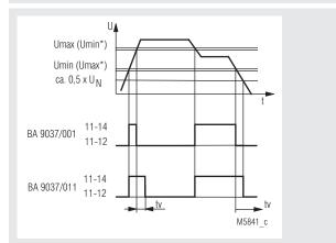
$^{\ast}$  U\_{\_{min}} and U\_{\_{max}} can also be exchanged. The hysteresis of the setting values is < 4 % of the response value
