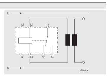
Connection Example with external galvanic seperation, e.g. by current transformer
