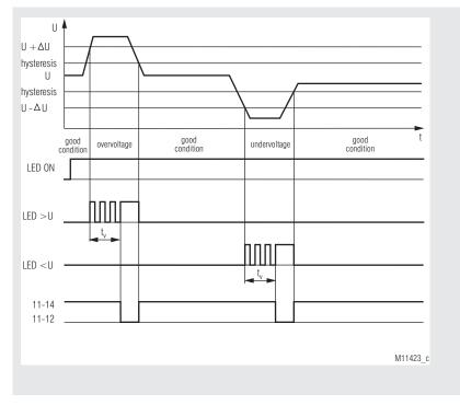
Monitoring function: voltage range; rotary switch: ",U<> "
