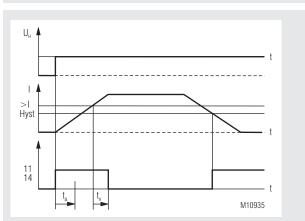
Example: overcurrent monitoring with de-energized on trip
