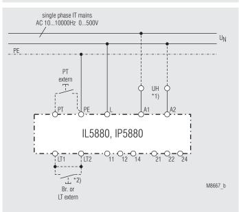
Monitoring of an ungrounded voltage system.
