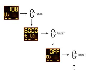
The default values set in the parameters (see parameter table) can be individually adjusted with the  $\bigvee \blacktriangle$  buttons; however, they must be within the respective setting ranges. The next parameter can be selected with the RUN/SET button and also be adjusted with the  $\bigvee \bigstar$  buttons.
