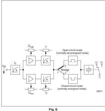
Simplified block diagram of a voltage measuring relay
