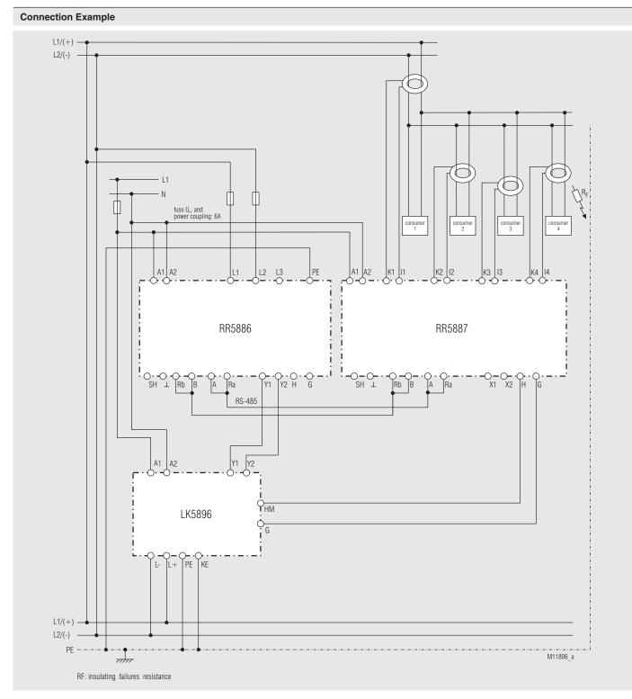
Insulation monitoring and insulation fault detection with 4 connected current transformers in a AC (DC)- network with subdistribution - insulation fault detection can be controlled by the insulation monitor /LK 5896); ALARM MEMORY active, i.e. alarm states are stored; bus termination of the first and last device on the RS-485 bus.
