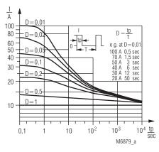
Diagram for short-time overload of the current input L1/i-L1/k (0.5  $\dots$  10 A)
