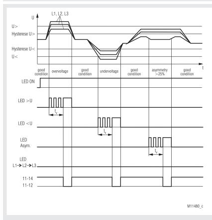
Monitoring function: 3 AC / 1 AC-overvoltage / undervoltage; rotary switch: "U>" / "U<"
