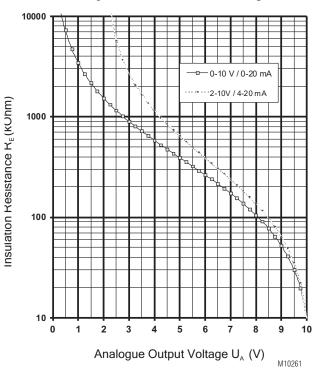
Analogue output voltage is proportional to the insulation resistance  $R_{_{\rm F}}$
