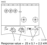
The adjustment of the unit can be made without additional measuring equipment and calculations. Please make sure that the load values are in the permitted operating range of the unit. Based on the max permitted values the BH 9097 can be used for 48 kW 3-phase motors at 3 AC 690 V and 5.8 kW single phase motors at AC 230 V.
