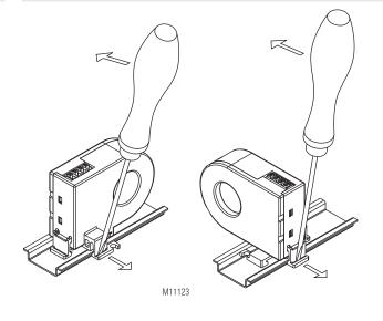
Disassembling Residual Current Monitor ND 5015/070
