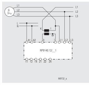
For 3-phase connections with current transformer (external).
