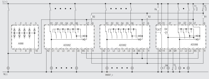
T1 external pushbutton for lamp test T2 external acknowledgement pushbutton for lamp signal T3 external acknowledgement pushbutton for audible alarm R<sub>v</sub>, R1, R2 > DC 30 V
