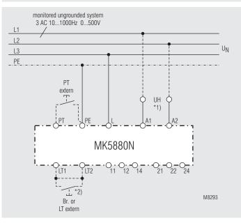
Monitoring of an ungrounded voltage system.
