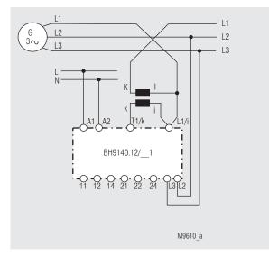
For 3-phase connections with current transformer (external).
