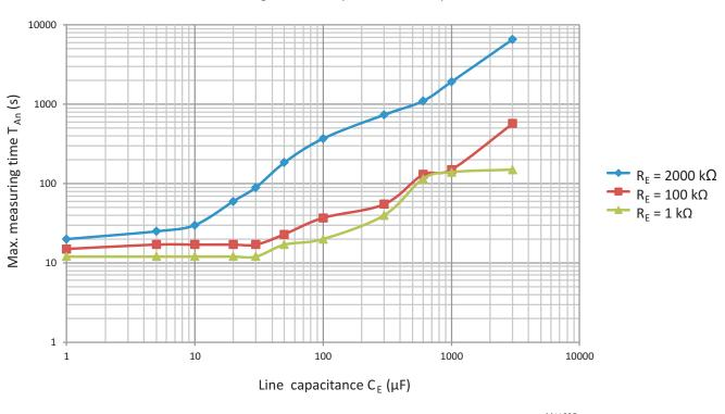
Max. measuring time in response to line capacitance
