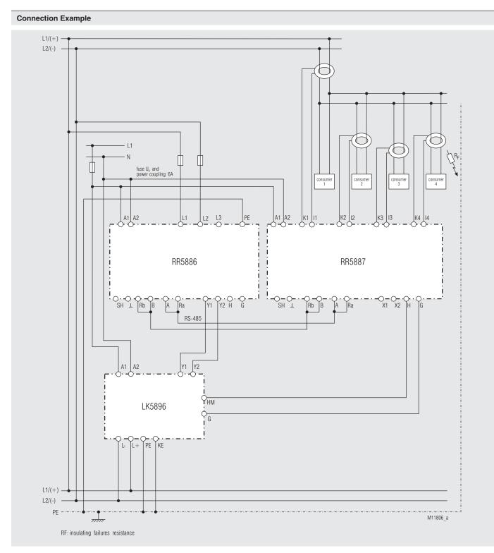
Insulation monitoring and insulation fault detection with 4 connected measuring current transformers in a AC (DC)- network with subdistribution - insulation fault detection can be controlled by the insulation monitor /LK 5896); ALARM MEMORY active, i.e. alarm states are stored; bus termination of the first and last device on the RS-485 bus.
