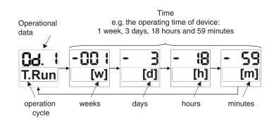
All operational data is deleted by pressing "Mode" and "Test" for more than 2 seconds in operational data display mode. The reset is confirmed on the display "ResOd" (Reset operational data).
