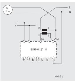
For single or 3-phase connections with current transformer (external)
