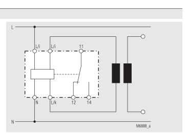
Connection Example with external galvanical seperation, e.g. via current transformer.
