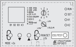
Wrong or contradictory entries of parameter values are recognised and displayed by the device as errors (setup errors). The error status can be exited by pressing the RUN/SET button longer than two seconds. The faulty parameters can be corrected back in the input mode.
