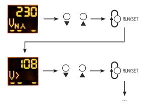
After the desired changes have been made, the new values are saved by pressing the RUN/SET button (> 2 s).
