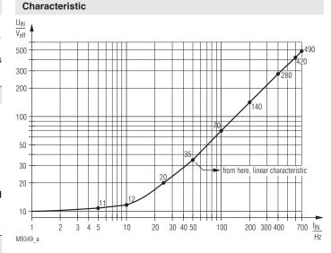
Typical sensitivity of the measuring input at variant MK 9837N.12/\_5\_
