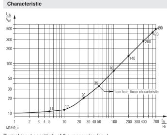
Typical input sensitivity of the measuring input with variant IL 9837.11/500  $\,$
