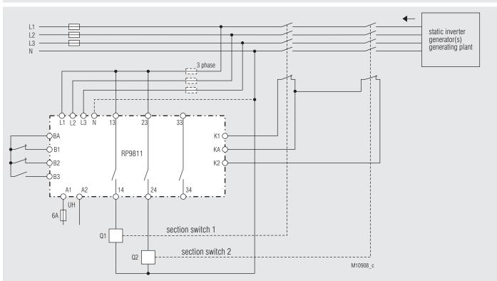
Application example according to DIN VDE-AR-N 4105 (from 30 kW); CEI 0-21 (from 20 kW); BDEW-directive; DIN V VDE V 0126-1-1 2 section switches
