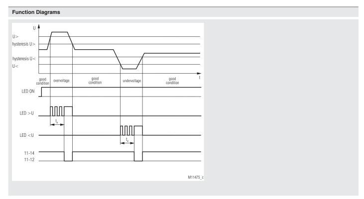
Monitoring function: overvoltage / undervoltage; rotary switch: "U>" / "U<"
