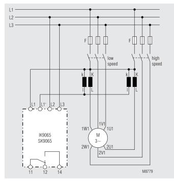
IK/SK 9065.11 for motors with separate windings
