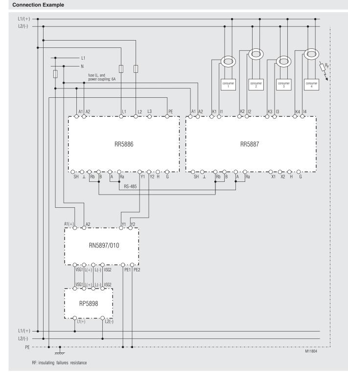
Insulation monitoring and insulation fault detection with 4 connected current transformers in a DC/AC network with subdistribution - insulation fault detection can be controlled by the insulation monitor (RN 5897/010); bus termination of the first and last device on the RS-485 bus.
