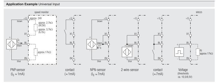
Note: For IK-models the auxiliary voltage (DC 24 V) must be additionally connected to terminals +U/0V
