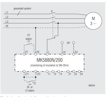
Monitoring of motorwindings againgst ground The insulation of the motor to ground is monitored as long as contactor K
