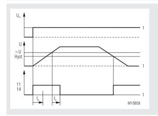
Example: overvoltage monitoring with closed circuit operation
