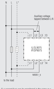
\*) a second fuse can be monitored in the same or a different phase via the terminals L1-L1
