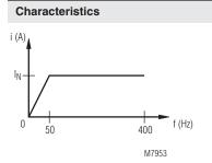
Max. input current curve in relation to input frequency
