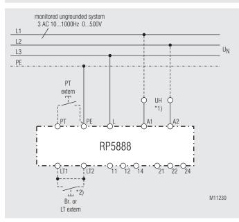
Monitoring of an ungrounded voltage system.
