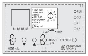
To change the parameters manually, the RUN/SET button must be pressed longer than two seconds. The display mode is accessed. The input mode is accessed when subsequently pressing " $\mathbf{\nabla} \mathbf{A}$ ". The input mode is also accessed by turning one of the two rotary switches.
