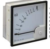
The indicating device EH 5861 is externally connected to the insulation monitor on terminals UA / GA (0 - 10 V) and shows the actual insulation resistance of the voltage system to ground. Dimensions: Width x heigth x depth 96 x 96 x 52 mm
