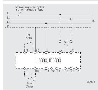
Monitoring of an ungrounded voltage system.
