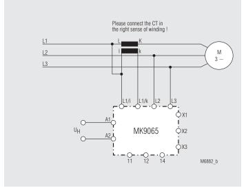
Connection Example for MK 9065.11 with current transformer
