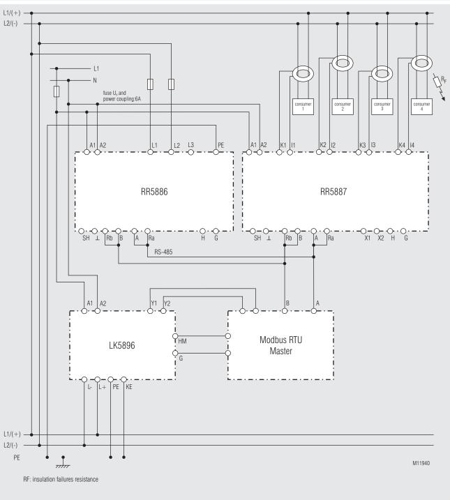
Modbus control insulation fault detection with external bus master
