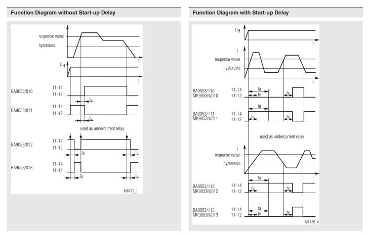
On model BA 9053/6\_ \_ with manual reset the contacts remain in the fault state after detecting a fault or after to has elapsed. The contacts are reset by disconnecting the supply voltage.
