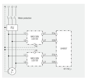
Inverter monitoring function, 3-phase with frequency monitor UH 6937
