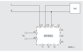
Connection Example for MK 9065.11 with single phase connection
