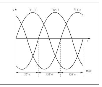
Fig. 2: Sinusoidal time characteristic
