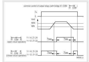
common control of output relays
