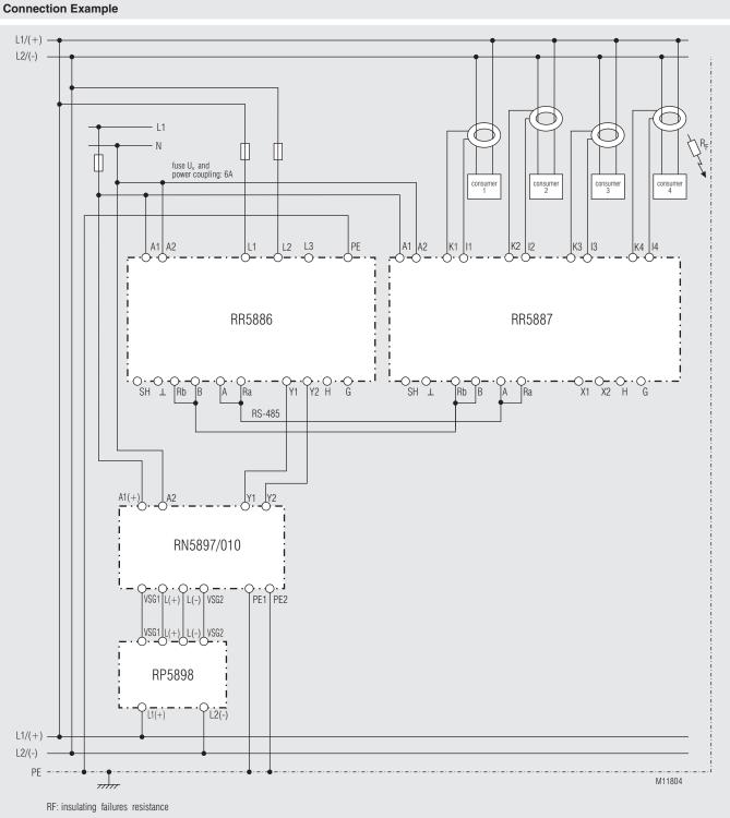
Insulation monitoring and insulation fault detection with 4 connected current transformers in a AC (DC)- network with subdistribution - insulation fault detection can be controlled by the insulation monitor (RN 5897/010); bus termination of the first and last device on the RS-485 bus.
