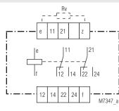
BA 9036 connection diagram for AC voltage
