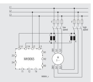
Connection Example for MK 9065.20 for motors with separate windings
