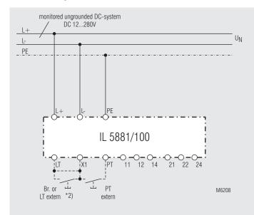
Monitoring of an ungrounded system without auxiliary supply. \*2) with bridge LT - X1: automatic reset
