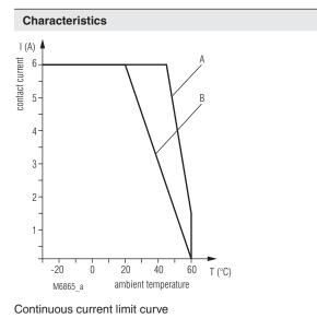
A = Devices mounted with 2 cm distance B = Devices mounted without distance
