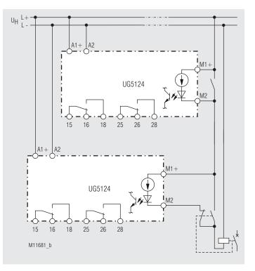
Trip circuit monitoring with NC and NO contact (auxiliary contacts) of the circuit breaker
