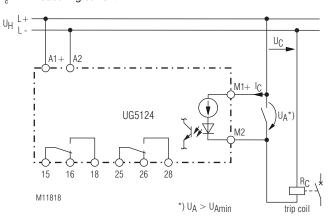
The voltage U<sub>Amin</sub> has a hysteresis of 2 %. I.e. the relay switches at a voltage of U<sub>Amin</sub> - Hysteresis in error state (contacts 15, 16 and 25, 26 closed). If the voltage U<sub>Amin</sub> is acceded, the relay switches to good stated (contacts 15, 18 and 25, 28 closed).
