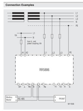
3AC network with manual test current output; EDS measuring bus connection without bus termination
