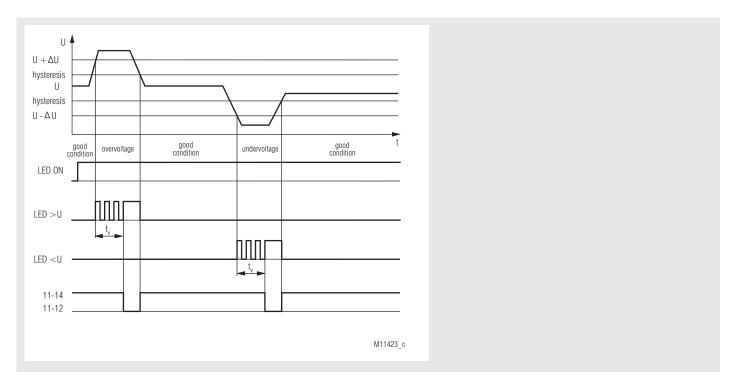
Monitoring function: voltage range; rotary switch: "U<>"
