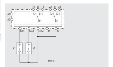
Application as contact protection relay, e.g. for two reed contact switches (K1, K2).
