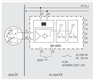
Thermistor motor protection relay shown as variant MK 9003/\_1\_ \_ , with safe separation according to EN 61 140, EN 60 947-1, 6 kV/2 between:
