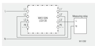
Noise filtering in a single wire with max. current capacity 50 mA
