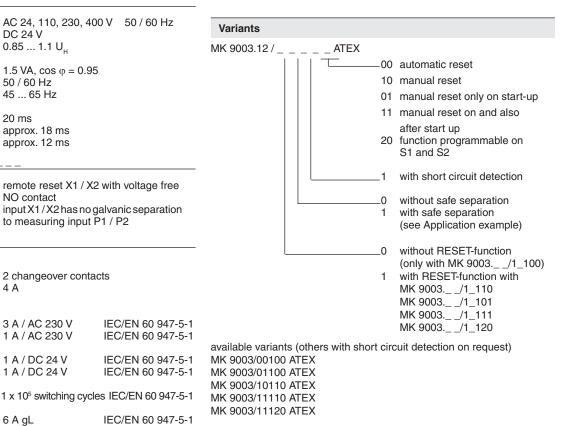
**Ordering Example for Variants** ATEX AC 230 V 50 / 60 Hz MK 9003.12 / Nominal frequency Auxiliary voltage Variant Contacts Туре
